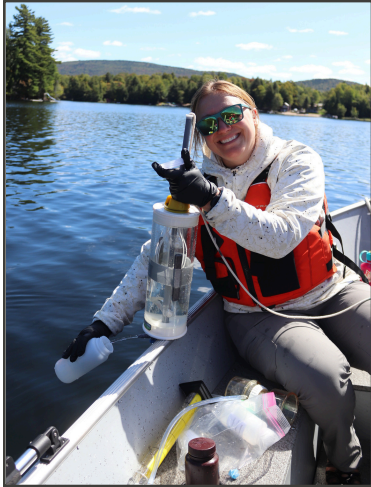
District technician Katie Whitkovits uses a Kemmerer Water Sampler to collect lake water for analysis.
