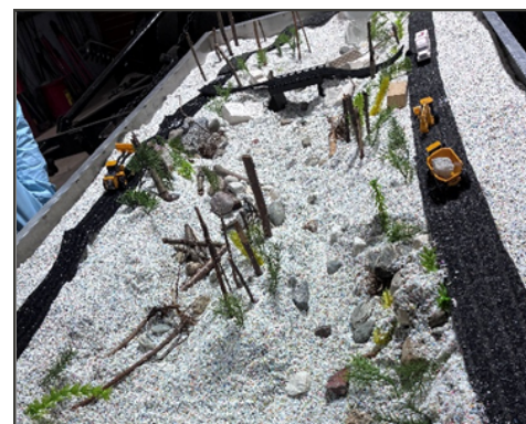
Stream tables simulating undersized culverts and practices that protect our roads.
